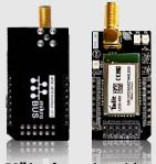
"tRF BoB 50" is a formative with a microBUS structure. It is an effective and easy solution for adding 868 MHz RF communication to vour design.It features the Telit LE50-868MHz transceiver module, a SMA connector for an antenna also two radio communication(Tx - Rx) LEDs. tBoB RF 50 communicates with the target board microcontroller via microBUS UART (Rx, Tx), AN, RST, PWM and INT lines. It has a LED diode in order to power indicator.
