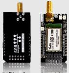
"tRF BoB 51" is a formative with a microBUS structure. It is an effective and easy solution for adding 868 MHz SIGFOX RF communication to your design.It features the Telit LE51-868MHz transceiver module, a SMA connector for an antenna also two radio communication( Tx - Rx ) LEDs. "tBoB RF 51" communicates with the target board microcontroller via microBUS UART ( Rx, Tx), AN, RST, PWM and INT lines. It has a LED diode in order to power indicator.
