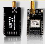
"tGPS BoB" is a formative with a microBUS structure. It is an effective and easy solution for adding GPS functionality to your design.It features the Telit SL869 - V2S module, a SMA connector for an GPS antenna also it has two LEDs for PPS and PWR. tGPS BoB can be interfaced with the target board microcontroller via microBUS UART (Rx, Tx), lines. It has a LED diode in order to power indicator.it can function on 3.3 V power supply only.
