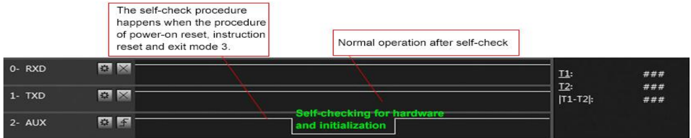
Timing Sequence Diagram of AUX when self-check
