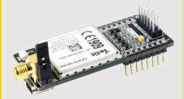
"t910 BoB" is a formative with a microBUS structure. It is an effective and easy solution for adding GSM/GPRS/3G solutions into your design. It features the Telit GE910-QUAD or UE910-EUR module, a SMA connector for an antenna, a SIM CARD socket. t910 BoB communicates with the target board microcontroller via microBUS (Rx, Tx, Rx2, Tx2, RTS, CTS, Reset, GPIOs). The Audio Connector is compatible with Iphone, Samsung, HTC headsets. It has two LED diodes for power indicator and status.
